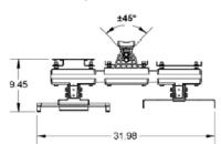
PTS5G-BK5132-HP2P **Specifications** Material Powder Coated Aluminun Hardware Material Stainless Steel Color Light Textured Gray Dimensions See Outline Drawings Unit Weight 25.3 lbs Mechanical Azimuth for Bracket +/- 45° Wind Survivability 175 mph
