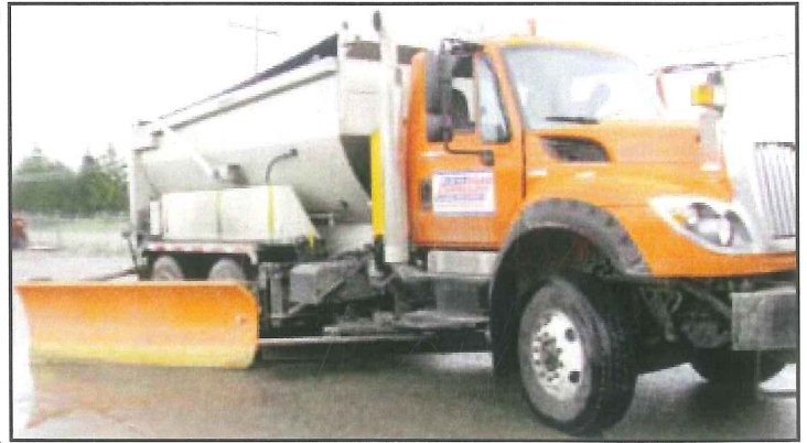
An RCOC plow truck equipped with a wing plow.
